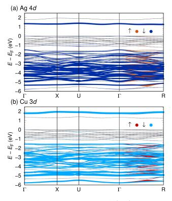
FIG. 2. GGA+U band structure of CuAg(SO<sub>4</sub>)<sub>2</sub> in the lowest energy AFM state. Colors red (spin  $\uparrow$ ) and blue (spin  $\downarrow$ ) indicate (a) Ag 4d orbital weights and (b) Cu 3d orbital weights. The altermagnetic property of CuAg(SO<sub>4</sub>)<sub>2</sub> is clear from the spin splitting along  $\Gamma$ -R path.
