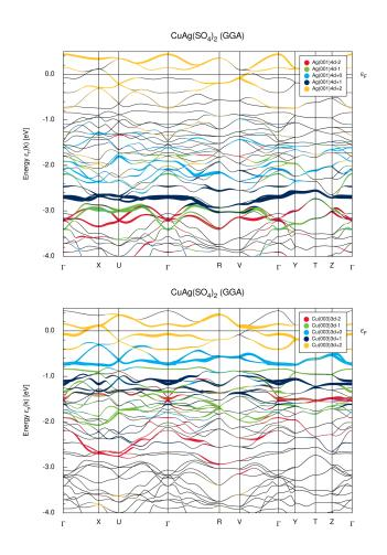
Figure S1. GGA band structure of CuAg(SO<sub>4</sub>)<sub>2</sub> with orbital weights of Ag (top) and Cu (bottom). Ag 4d and Cu 3d orbital character, respectively, are highlighted:  $d_{xy}$  (m = -2) red,  $d_{yz}$  (m = -1) green,  $d_{z^2}$  (m = 0) blue,  $d_{xz}$  (m = 1) dark blue,  $d_{x^2-y^2}$  (m = 2) yellow.
