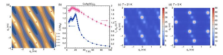
FIG. 5. Susceptibility and classical Monte Carlo results for  $\text{CuAg}(\text{SO}_4)_2$ . (a) Susceptibility  $\chi(\mathbf{q}, T)$  of  $\text{CuAg}(\text{SO}_4)_2$  at T = 300 K estimated using Eq. 4. (b) CMC specific heat and susceptibility. (c) and (d) correspond to spin structure factors at T = 21 K and T = 5 K, respectively. Note that for the  $\mathbf{q}$  vectors in (a), (c) and (d) we neglect the small monoclinic angle of 94° and the difference in a and c lattice parameters.
