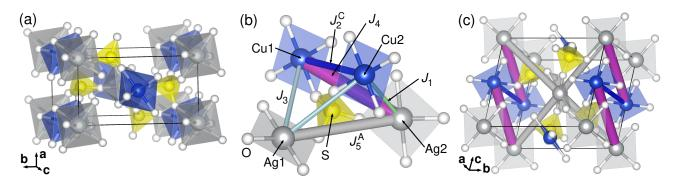
FIG. 1. (a) Crystal structure of  $\text{CuAg}(\text{SO}_4)_2$ , as reported in Ref. [8]. (b) Structural unit showing only one SO<sub>4</sub> cluster with its nearest neighbor connected via  $d_{x^2-y^2}$  orbitals. Cu and Ag sites are only numbered for use in Table II. (c) Illustration of relevant exchange paths in the structure of  $\text{CuAg}(\text{SO}_4)_2$ .
