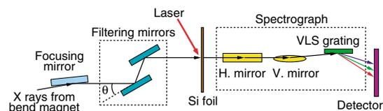
FIG. 1 (color online). Sketch of setup at ALS beam line 5.3.1.
