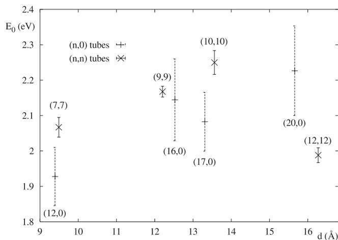
**FIGURE 2** Damage thresholds of single wall carbon nanotubes as a function of tube diameter. The duration of the laser pulse was  $\tau = 20$  fs. The + symbols and dashed error bars correspond to tubes of the  $(n, 0)$  type, the  $\times$  symbols and solid error bars to tubes of  $(n, n)$  type
